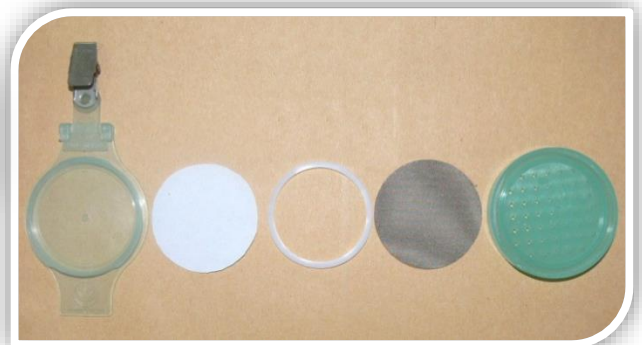
Schematic Diagram of diffusive passive samplers (a) and Lanwatsu passive samplers for \text{SO}_2 , \text{NO}_2 , \text{NH}_3 , \text{O}_3 (b) and for \text{HNO}_3 , \text{HCl} and carboxylic acids (c).
